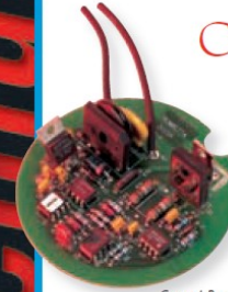
Current Regulating Over-Energizer (CROE)
